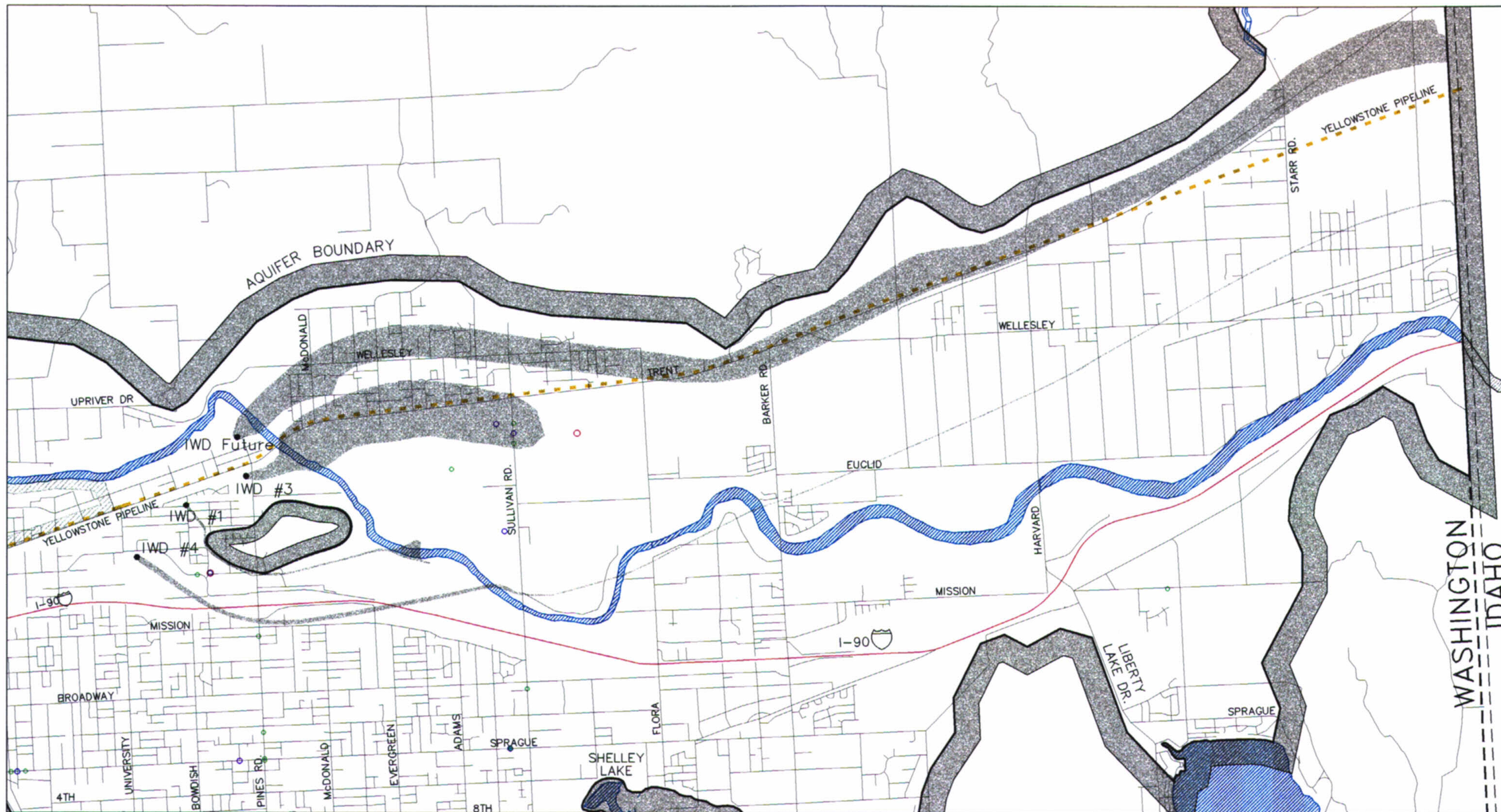
FIGURE 6-5B IRVIN WATER DISTRICT NO. 6 SPOKANE AQUIFER JOINT BOARD PROPOSED WELLHEAD PROTECTION AREAS AND POTENTIAL HISTORICAL CONTAMINANT SOURCES DECEMBER 1997
