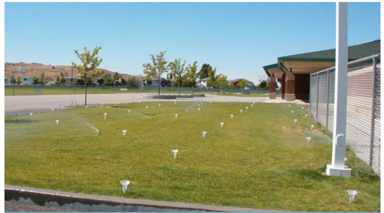
A catch can test is used to determine how long to run an irrigation system and how well the water is distributed over the landscape.
